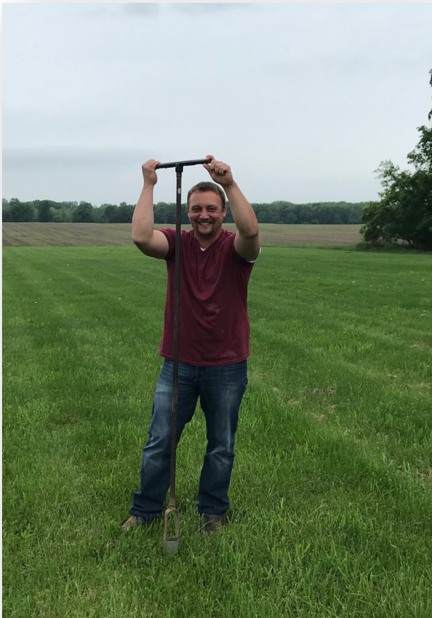
Above, Cody Johnson uses a soil auger to obtain a soil sample. This sample will be tested to gauge the suitability of the land for an on-site sewage system.
